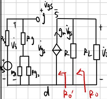
$$A_v = \frac{V_o}{V_i} = \frac{g_m v_{gs} R_L'}{v_{gs} + g_m v_{gs} R_L'} = \frac{g_m R_L'}{1 + g_m R_L'}$$
