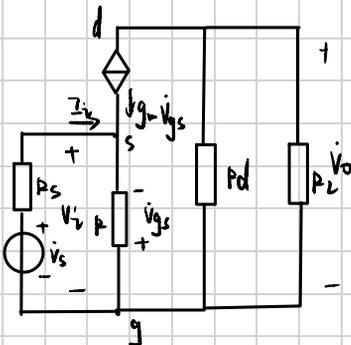
$$A_v = \frac{V_o}{V_i} = \frac{g_m v_{gs} R_L}{-v_{gs}} = g_m R_L$$
