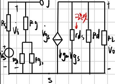
$$A_v = \frac{V_o}{V_i} = \frac{-g_m v_{gs} R_{d_s} \parallel R_L \parallel R_L}{V_{gs}} = -g_m R_L$$
