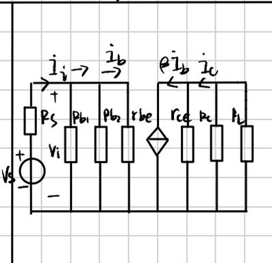
$$A_v = \frac{V_o}{V_i} = \frac{\beta I_b R_c \parallel R_L}{I_b \cdot r_{be}} = -\frac{\beta R_c'}{r_{be}}$$
