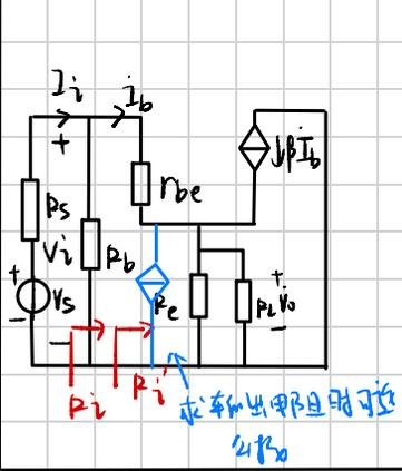
$$A_v = \frac{V_o}{V_i} = \frac{(1+\beta) I_b R_L'}{I_b [r_{be} + (1+\beta) R_L']} = \frac{(1+\beta) R_L'}{r_{be} + (1+\beta) R_L'} \leq 1$$
