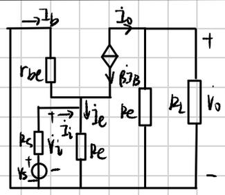
$$A_v = \frac{V_o}{V_i} = \frac{-\beta I_b R_L'}{-I_b r_{be}} = \frac{\beta R_L'}{r_{be}}$$
